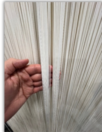
Membrane Bioreactor filters.
