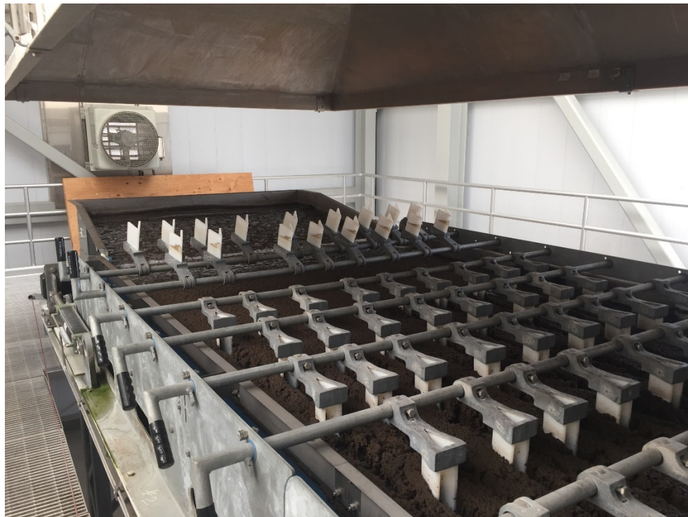
Figure 14.3. Gravity Drainage Section with Chicanes
